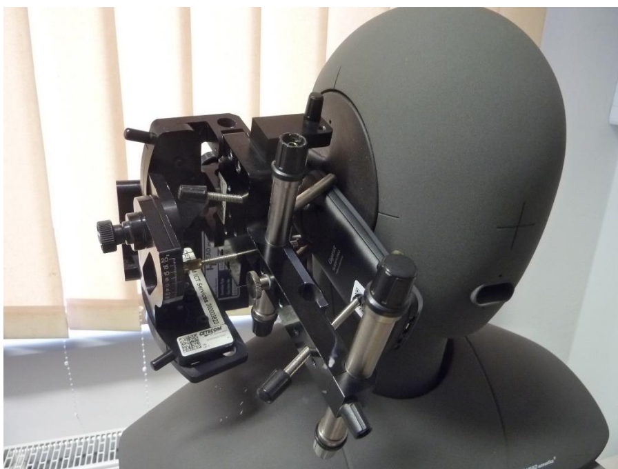
Photo 2: test setup for volume control (close-up view)
