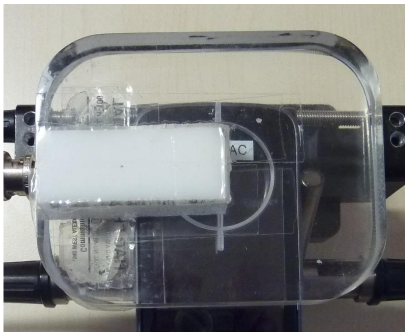
Photo 4: test setup for Radial field intensity (0 degree)
