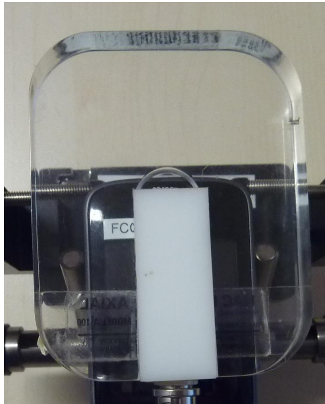
Photo 3: test setup for axial field intensity and magnetic field intensity frequency response
