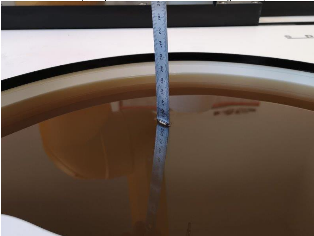
Photo 2: Liquid depth HBBL600-10000MHz Simulating Head Liquid
