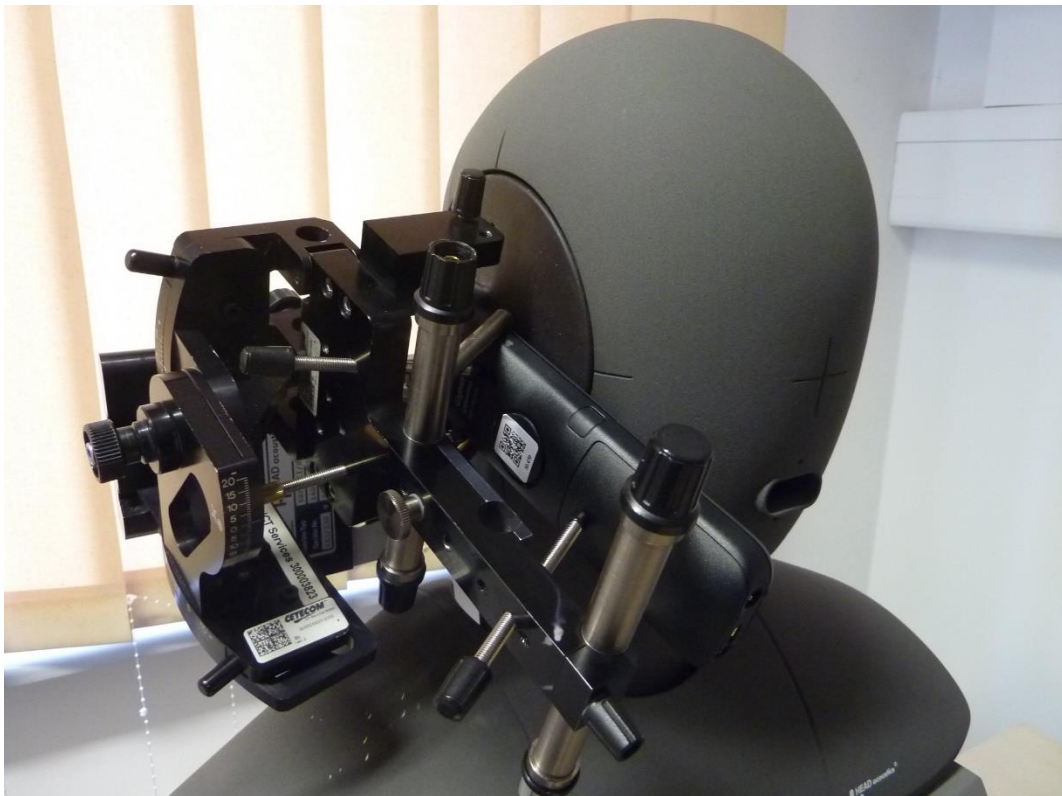
Photo 2: test setup for volume control (close-up view)
