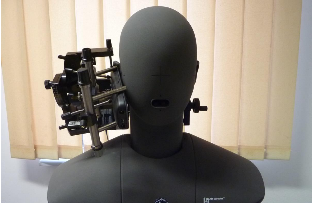
Photo 1: test setup for volume control
