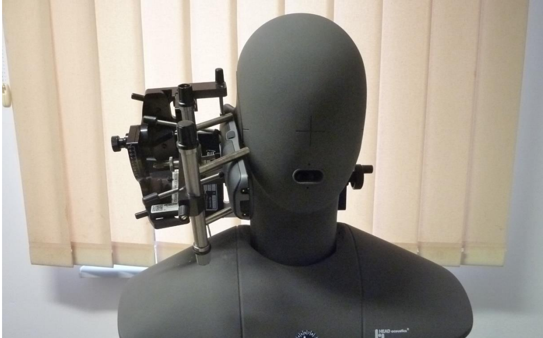
Photo 1: test setup for volume control
