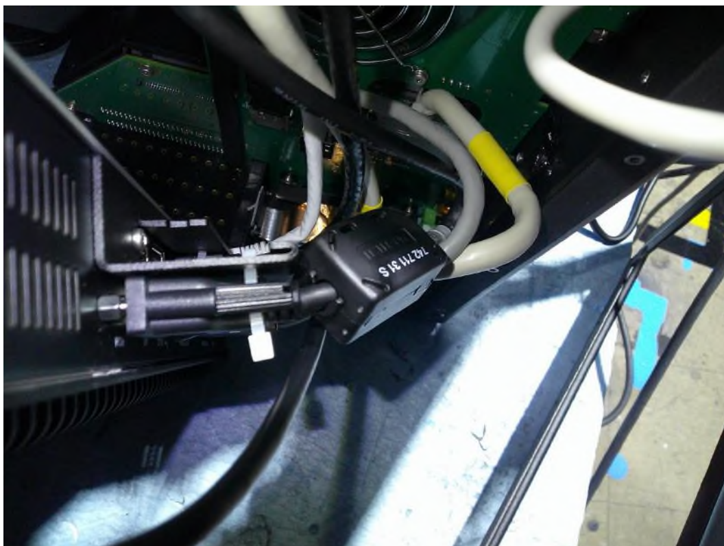
Photograph shows the ferrite fitted to the EUTs PCI connector. Wurth Elektronik part number 74271131S
