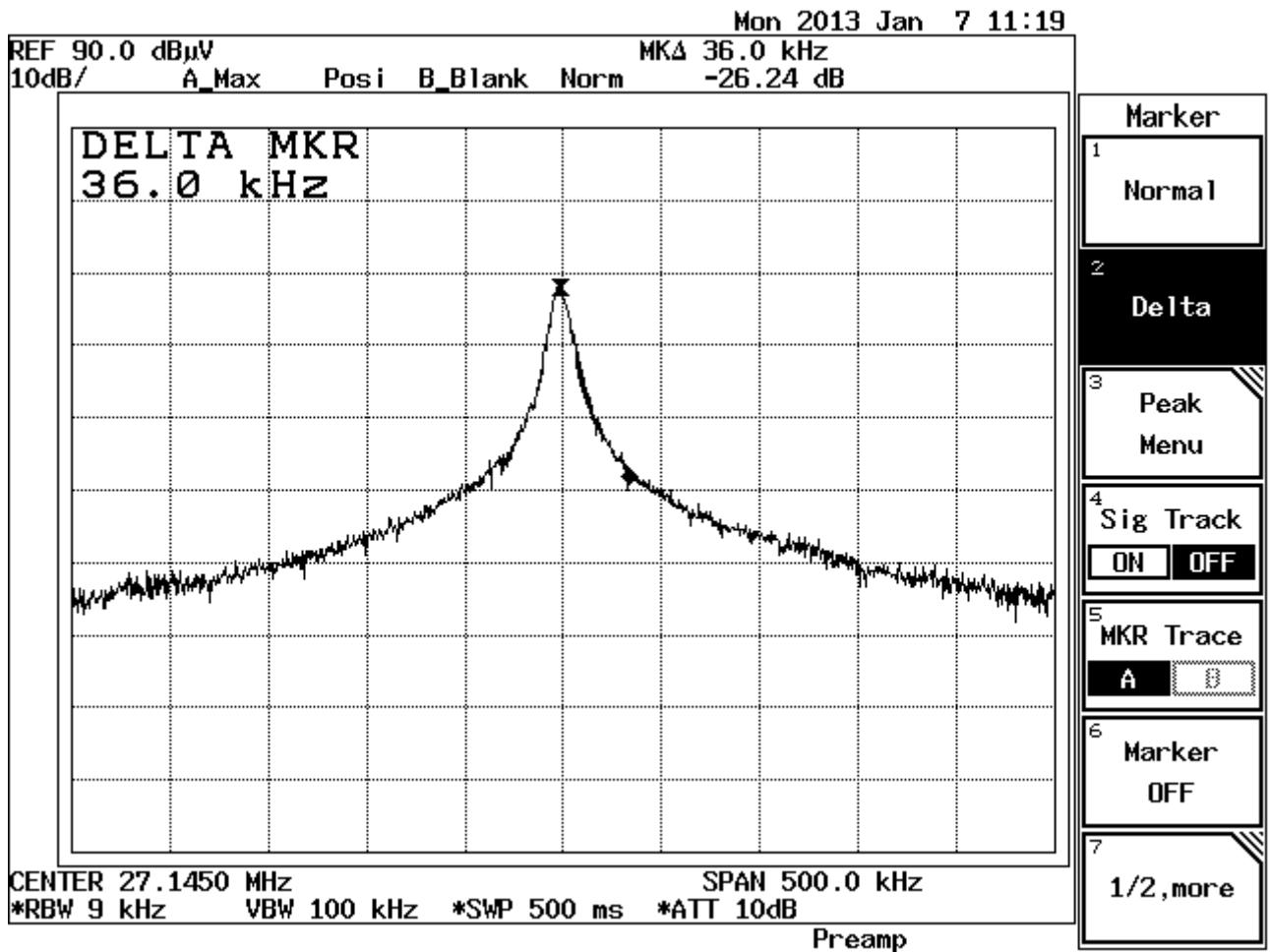
The field strength of any emission within the operation band did not exceed 80 dB( $\mu$ V/m) for average value or 100 dB( $\mu$ V/m) for peak value.
