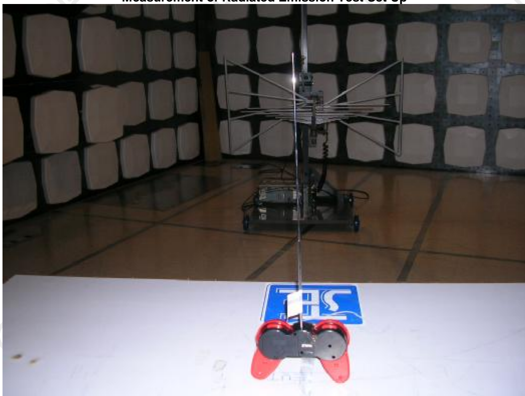
Measurement of Radiated Emission Test Set Up
