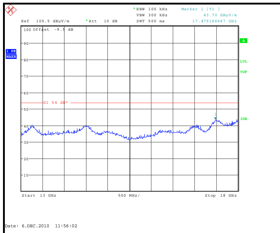
Receiver Radiated Spurious Emissions 13 GHz to 18GHz – 2405.0MHz
