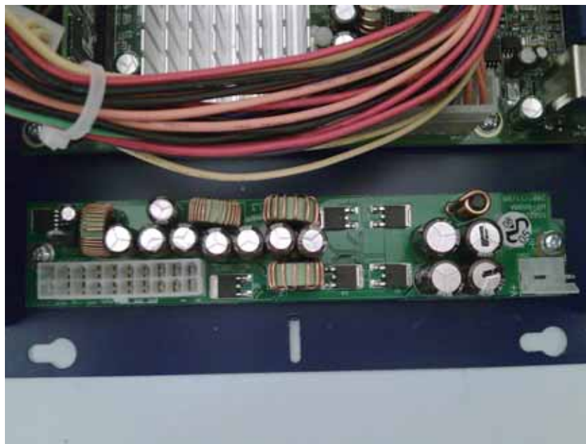
New Power Supply Mounted To Chassis Cables removed
