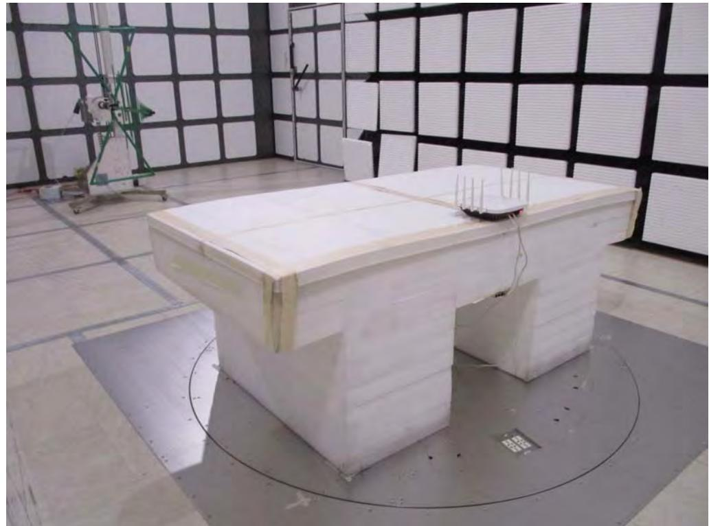
**Test Configuration: 1GHz~18GHz / Test Mode: Mode 1**
