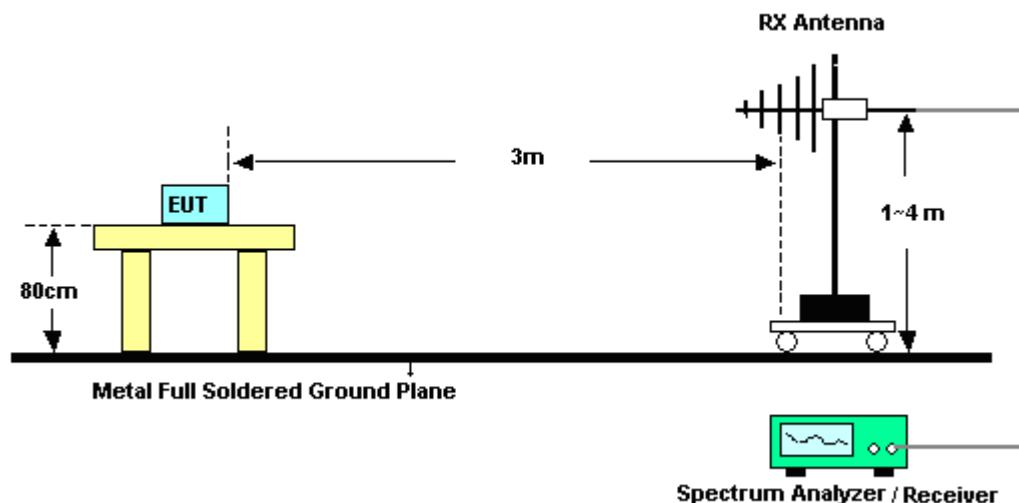
For radiated test from 1GHz to 18GHz
