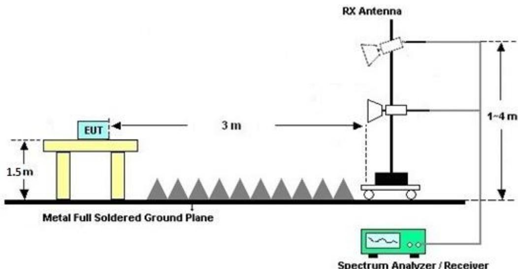
For radiated test above 18GHz
