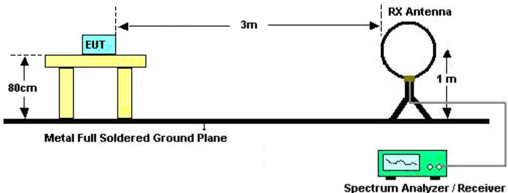
For radiated emissions from 30MHz to 1GHz
