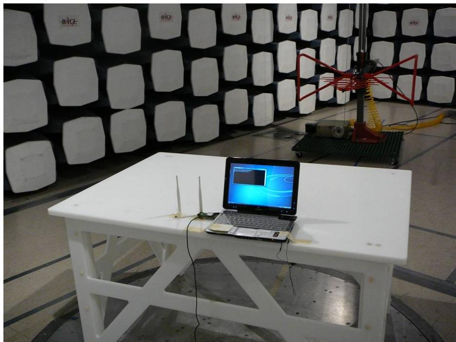
**9.3 Radiated Emission below 1 GHz Front View**
