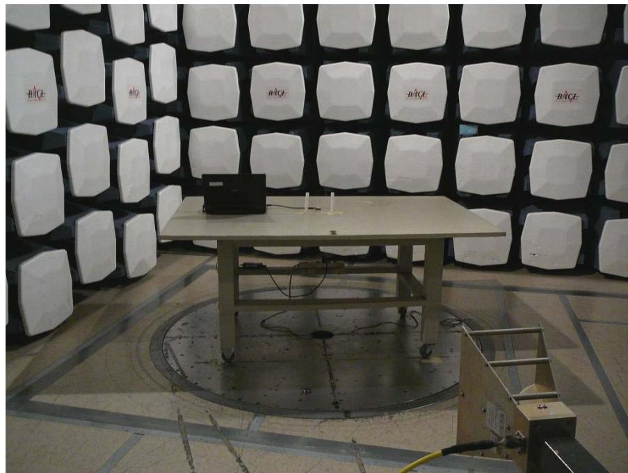
**15.4 Radiated Emission above 1 GHz - Rear View**
