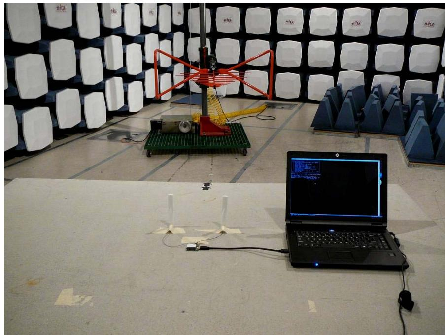
**15.3 Radiated Emission above 1 GHz - Front View**
