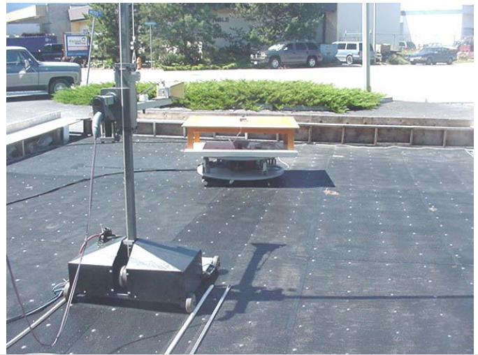
Photograph F.7-2 - Vertical 3115 Horn Cellular Radiated Emissions Setup
