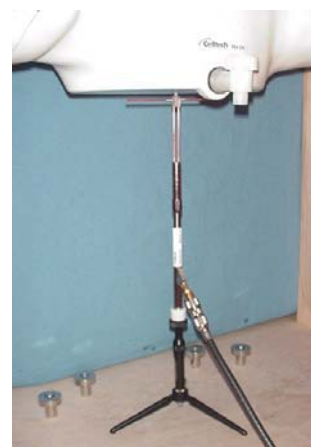
835MHz Dipole Setup
