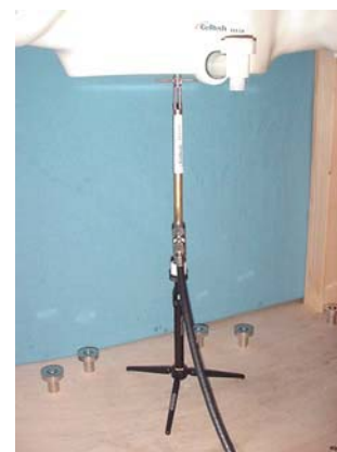
1900MHz Dipole Setup
