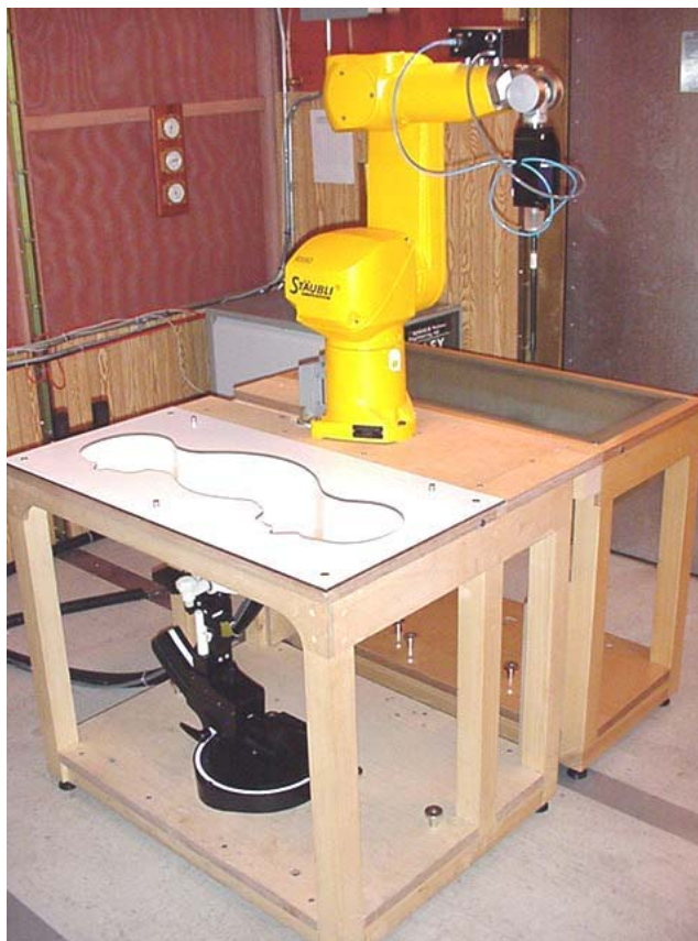
DASY4 SAR Measurement System with SAM phantom and device holder
