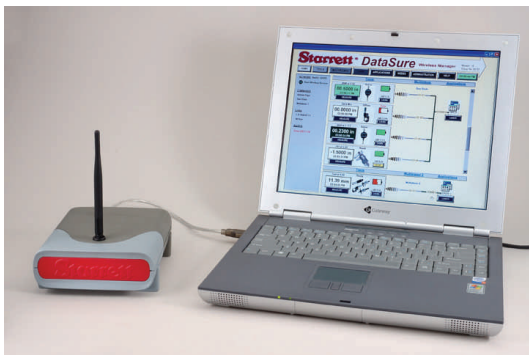
Figure 10 Gateway Connected to a Laptop Computer
