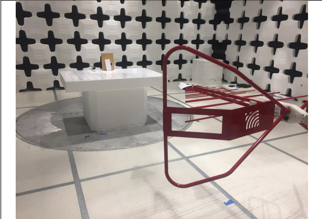
Radiated Emissions Below 1GHz setup – Front
