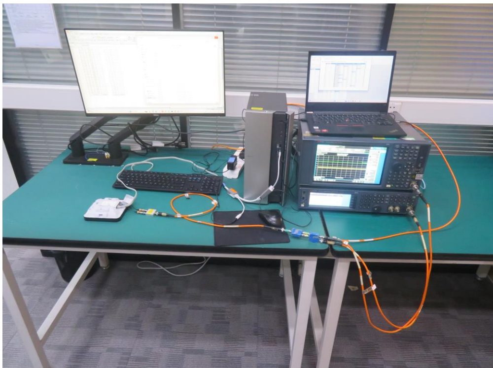
Description: Dynamic Frequency Selection Test Setup
