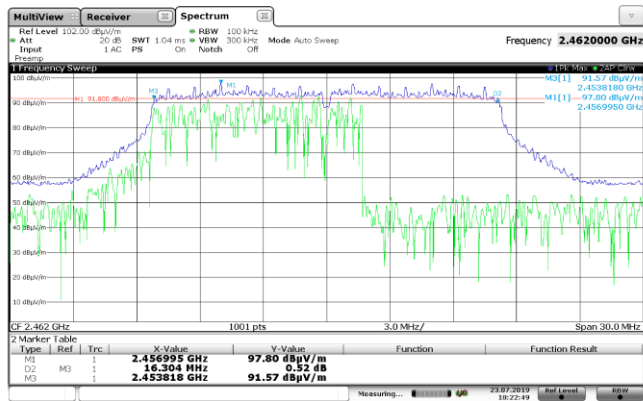
Figure 8.5-10: 6 dB bandwidth on 802.11g, sample plot
