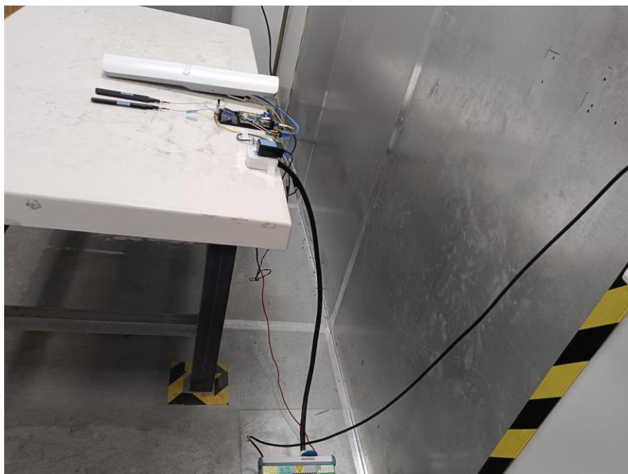
Description: Radiated Spurious Emissions Test Setup for below 30MHz
