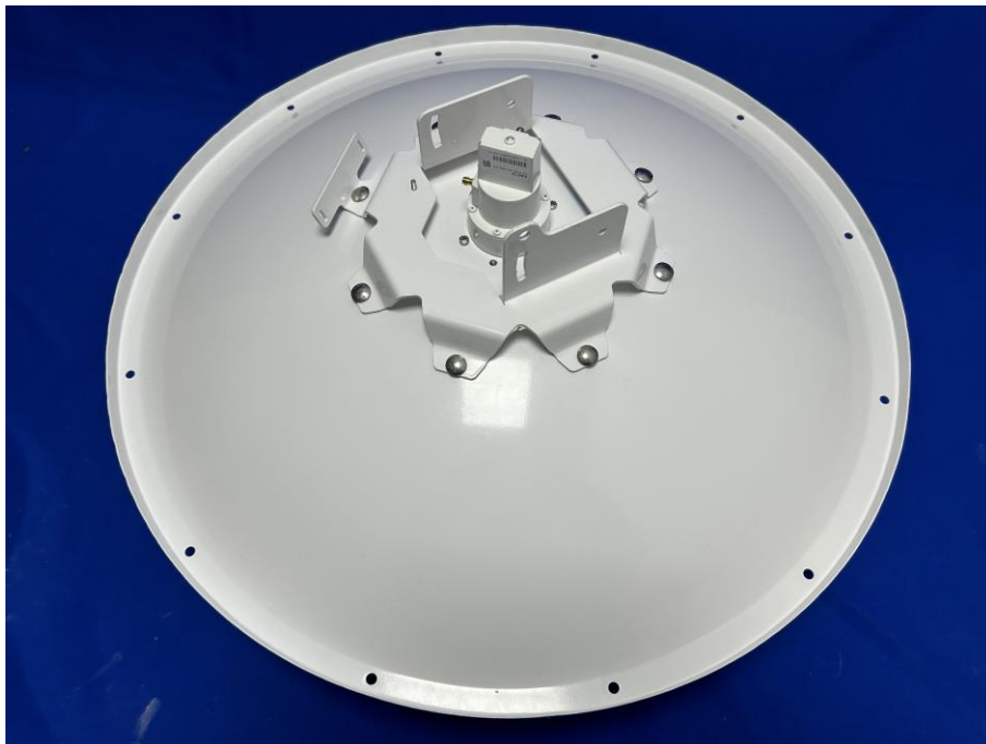
(6) Dish Antenna (MTAD-5G-30D3)
