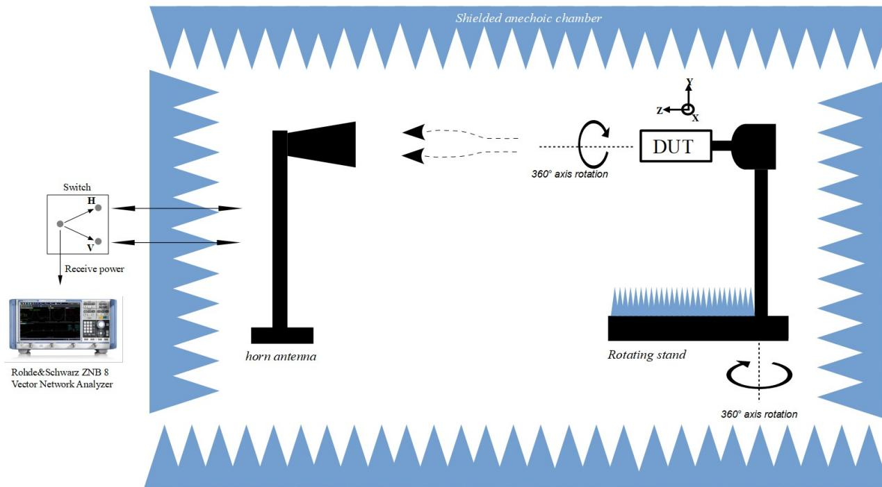
Explanation: Antenna testing is performed using the test setup above. Antenna gain is measured in 3d plane. The measurements are then taken and ran through CST studio Time domain solver simulation system to draw Antenna peak gain diagram. Simulation is performed taking into account pcb with components, case desing, heatsink and etc.
