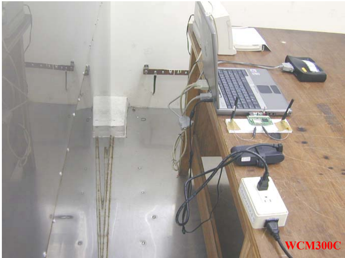
Photo 2: Conducted Emission Test Set-up
