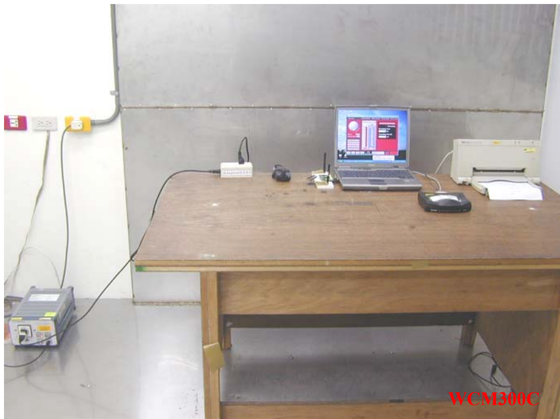
Photo 1: Conducted Emission Test Set-up
