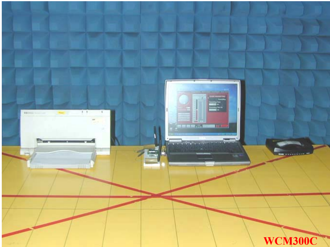
Photo 1: Radiated Emission Test Set-up
