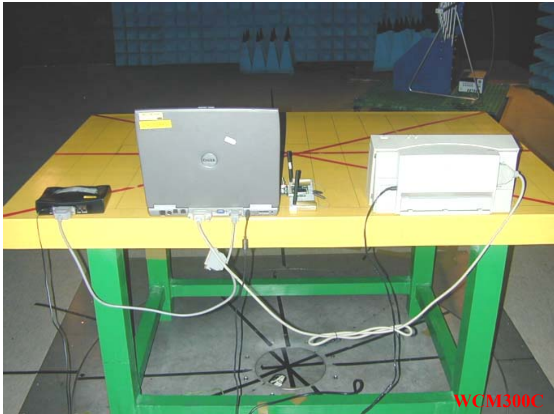
Photo 2: Radiated Emission Test Set-up
