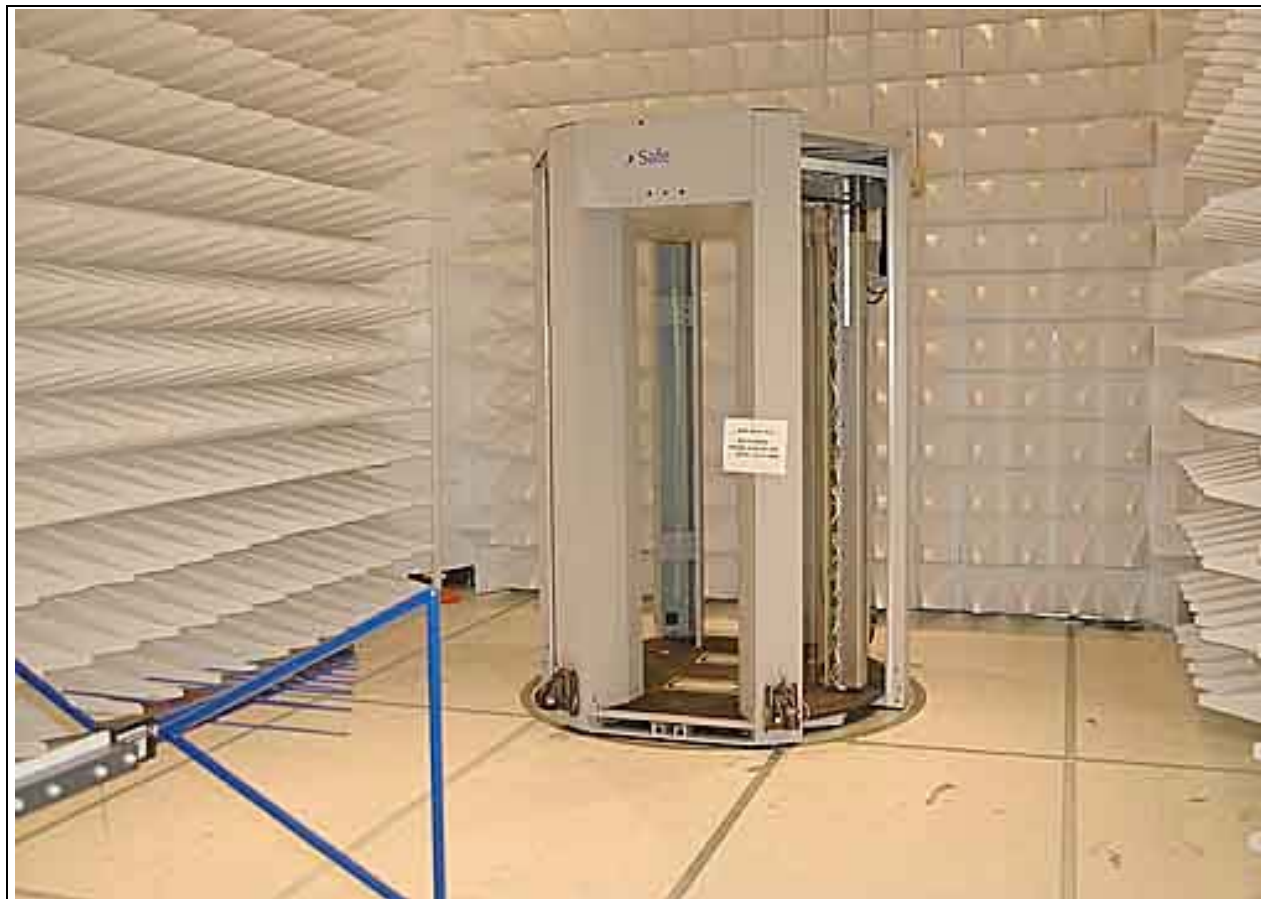
Radiated Emissions - Front View - 1-1000 MHz
