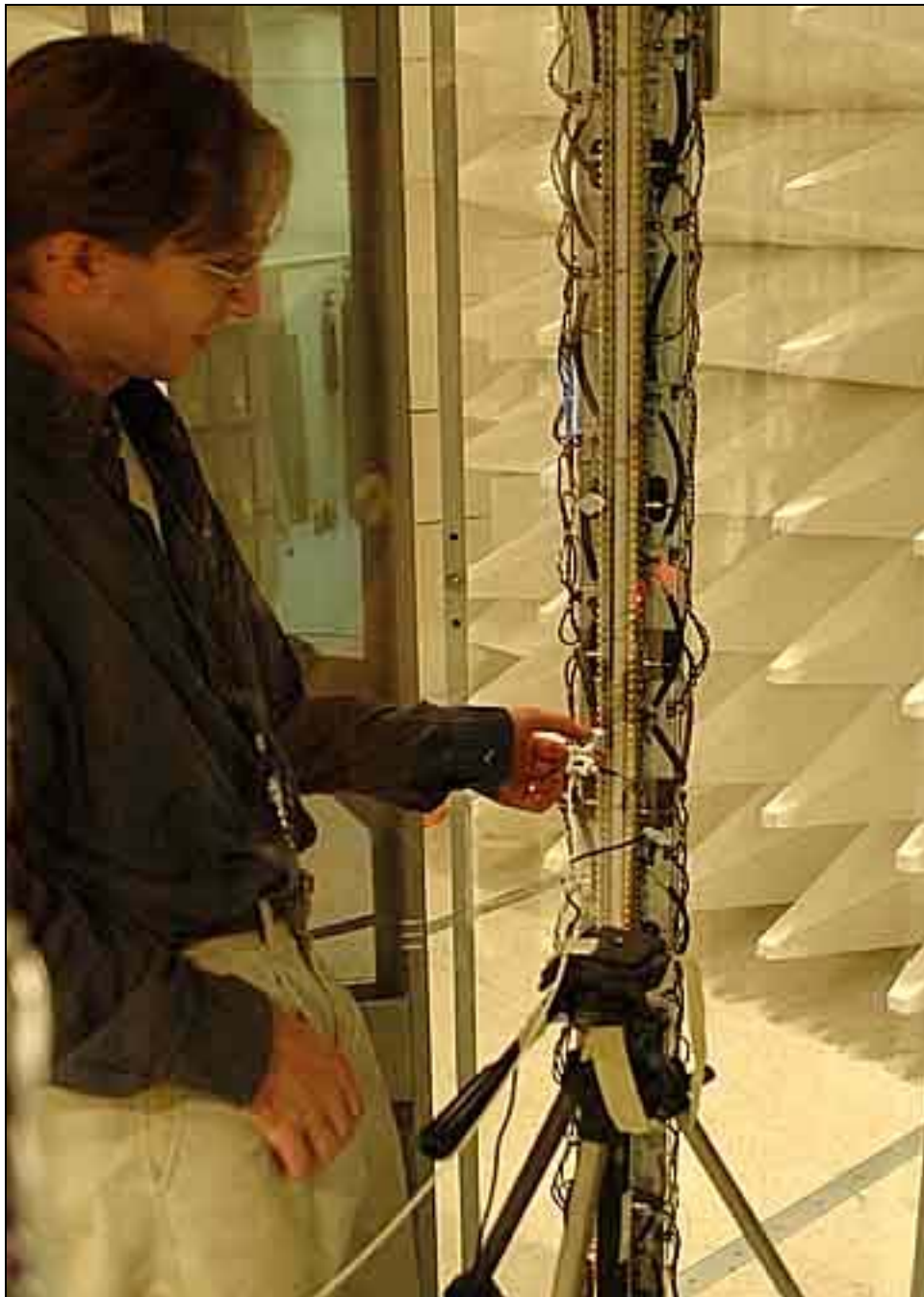
Radiated Emissions - 40-100 GHz Sample Setup Using Mixers
