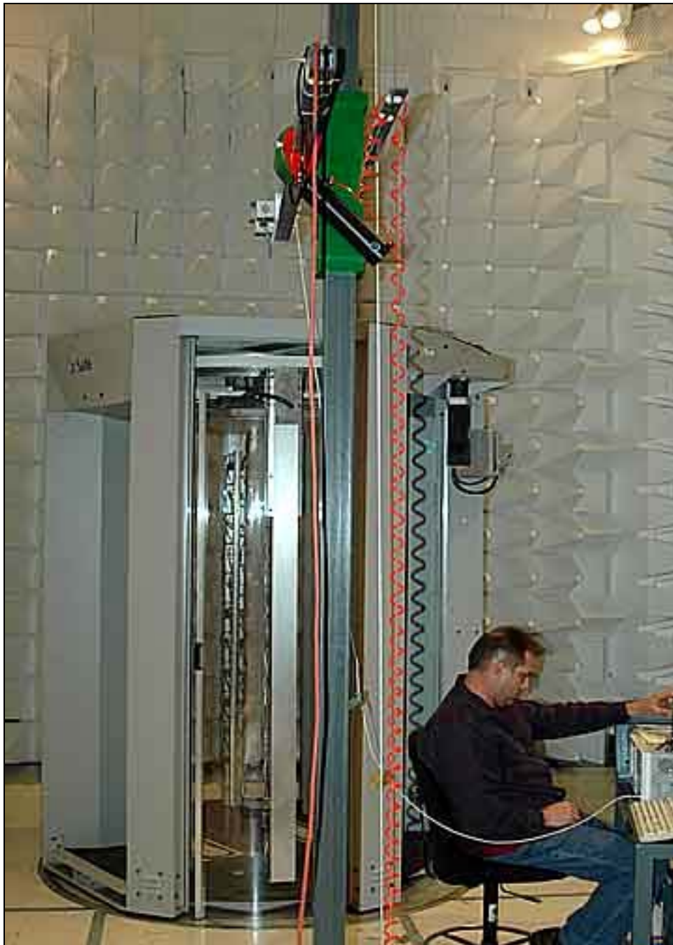
Radiated Emissions - 12-40 GHz Sample Setup at 3 Meters
