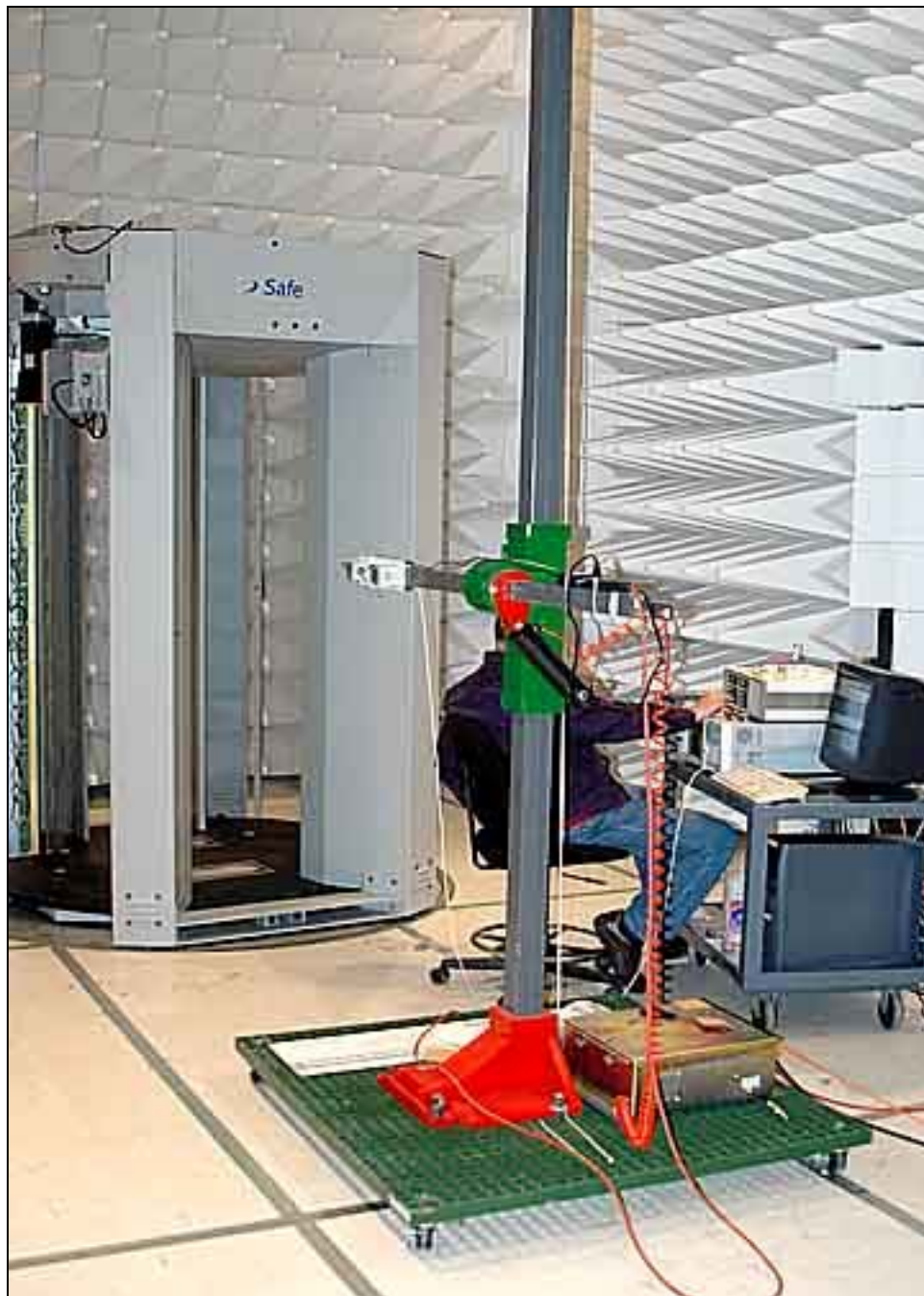
Radiated Emissions - 12-40 GHz Sample Setup at 1 Meter
