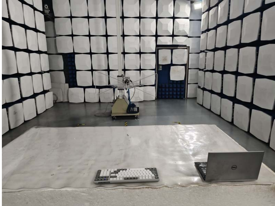
Radiated emission test view- Model: BK-7111
