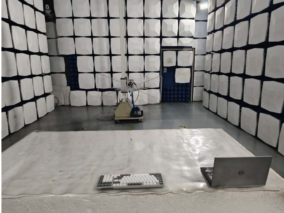
Radiated emission test view- Model: BK-7111
