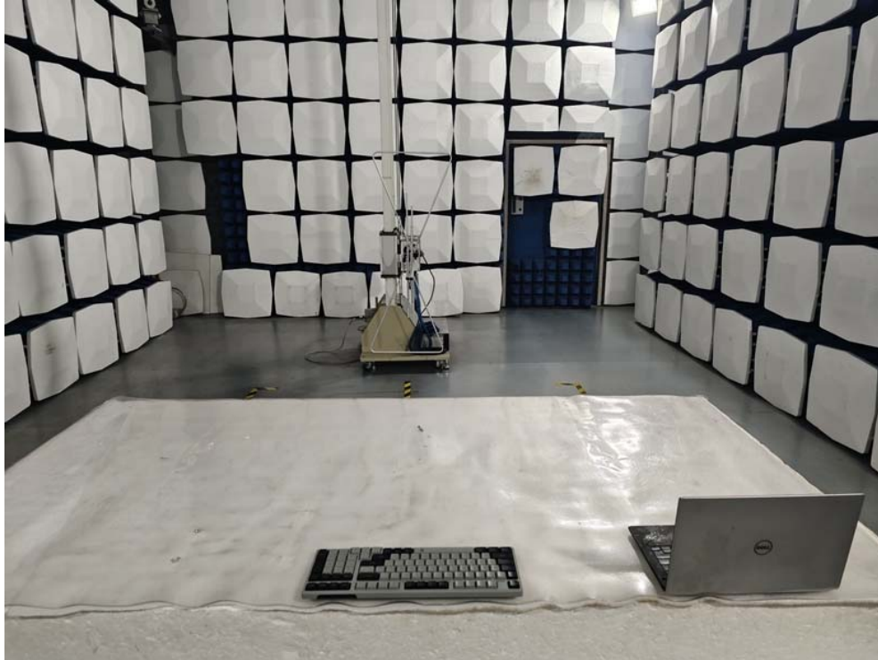
Radiated emission test view- Model: BK-7114WG
