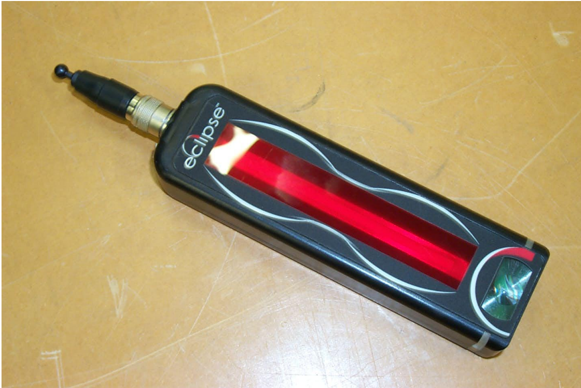
Figure 8 - Eclipse Laser Target, Front
