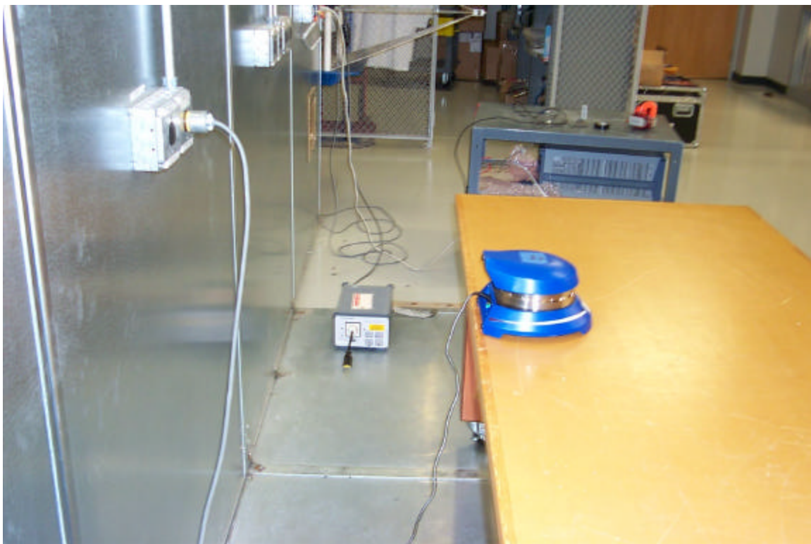
Figure 4 - Conducted Emissions Test Setup
