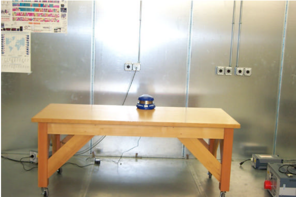
Figure 3 - Conducted Emissions Test Setup
