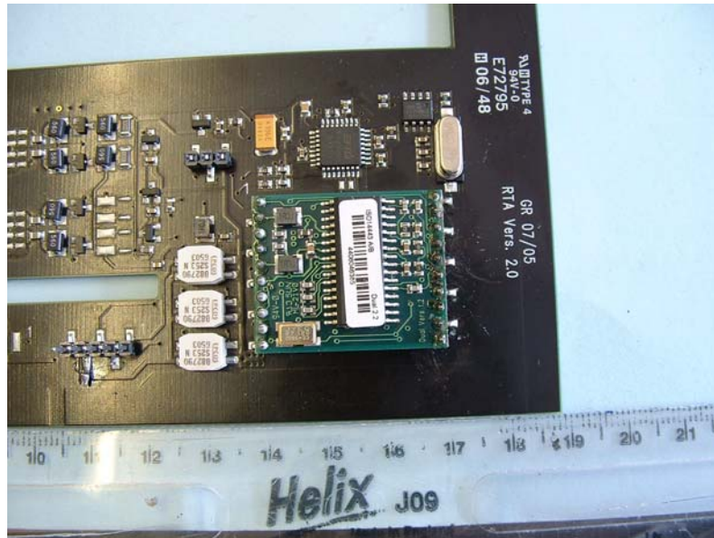
RF Module Mounted on Antenna PCB
