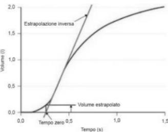
$$\text{Time zero} = t_{\text{PEF}} - (V_{\text{PEF}}/\text{PEF})$$
