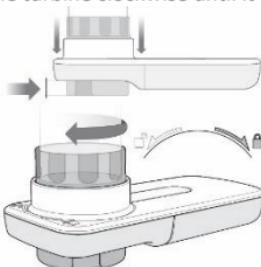
Insert the mouthpiece at least 0.5 cm into the turbine socket
