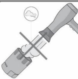
Correct functioning of the turbine is guaranteed only if it is "clean" and free of foreign bodies which interfere with its movement. The presence of dust or foreign bodies (such as hairs, sputum etc.) could slow or block the moving parts of the turbine and make the result less accurate, or damage the turbine itself. After each use, check the cleanliness of the turbine.
