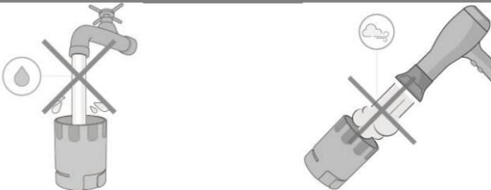
Correct functioning of the turbine is guaranteed only if it is “clean” and free of foreign bodies which interfere with its movement. The presence of dust or foreign bodies (such as hairs, sputum etc.) could slow or block the moving parts of the turbine and make the result less accurate, or damage the turbine itself. After each use, check the cleanliness of the turbine.
