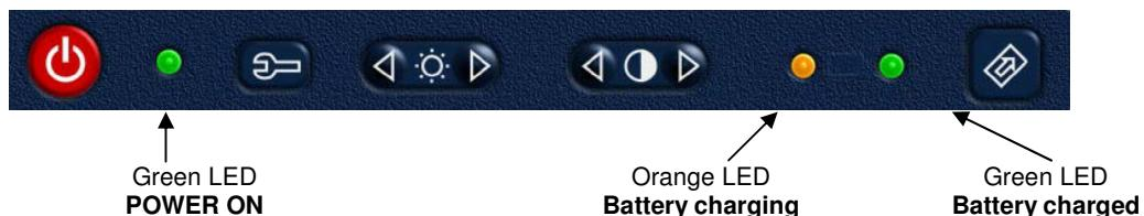
The charging process has several phases which are indicated by two LEDs, green and orange (as shown above).
