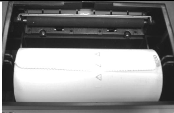
Push the paper into the slot located under the traction reel (black rubber reel).
