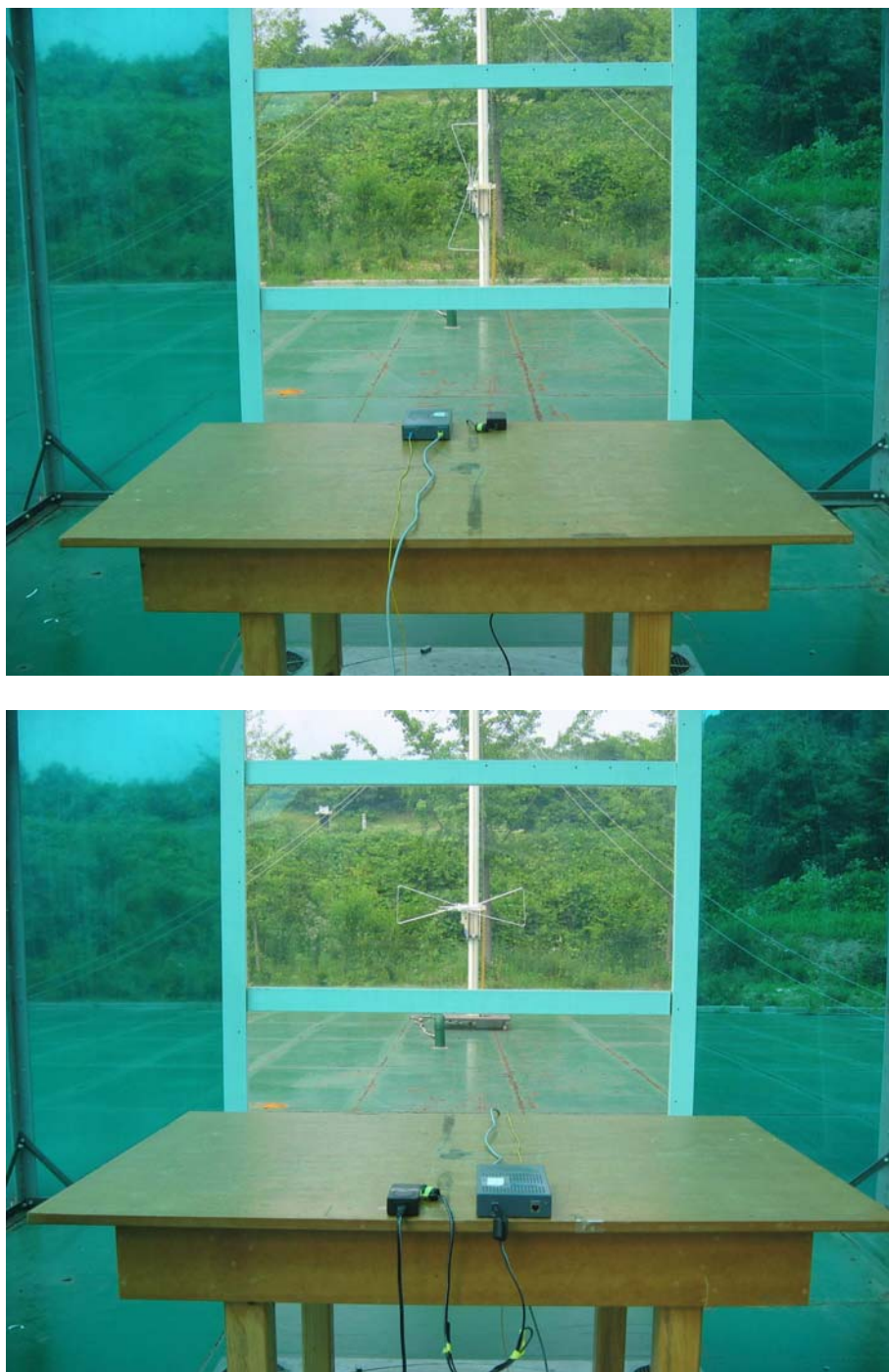
Figure 4. Photo of Radiated emission test setup
