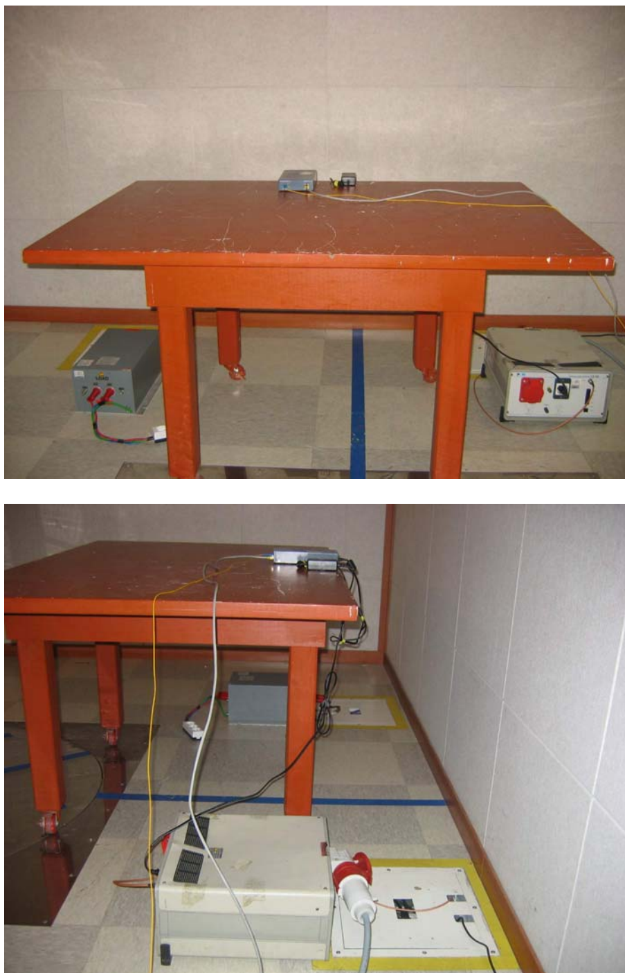
Figure 1 Conducted Emission Test Setup
