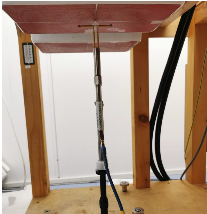
Figure 3 System check setup using a verification dipole
