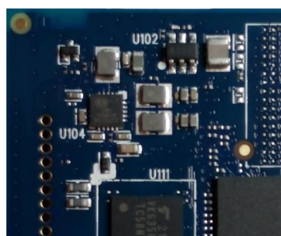
smaller AXP313A PMIC with additional DC/DC converters (on top and bottom)
