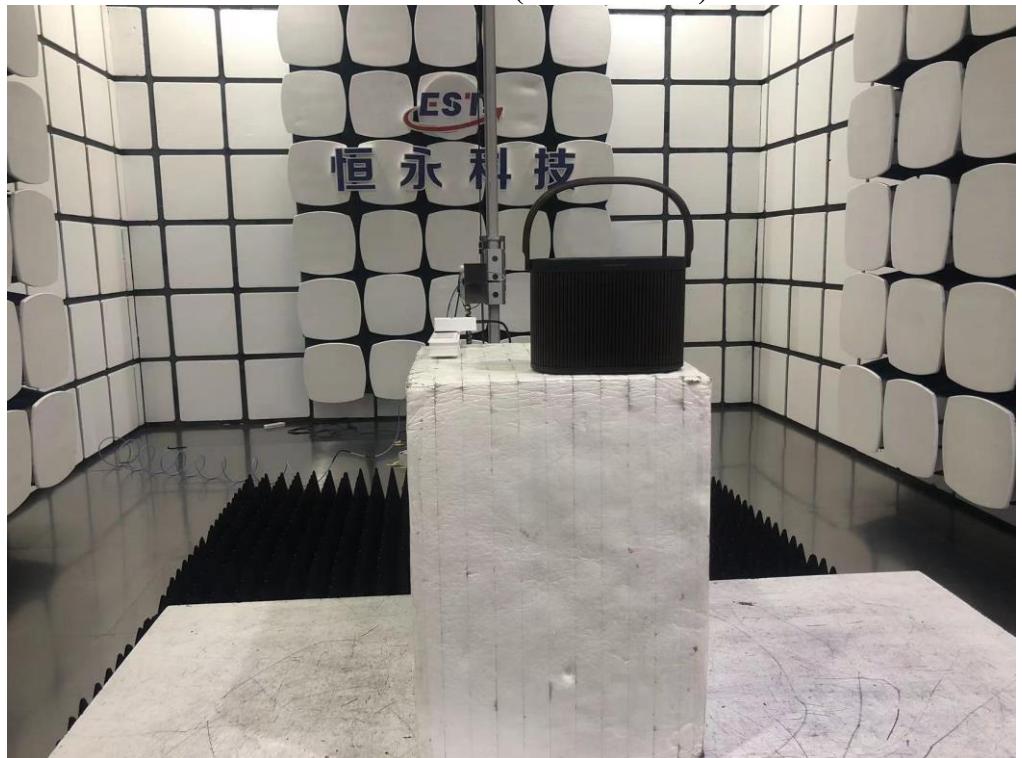
Radiated Test (Above 1GHz)
