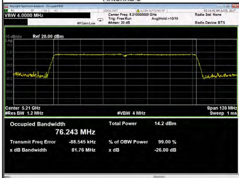
**IEEE 802.11ac 80 mode / 5290MHz****26dB Bandwidth****Antenna 0**
