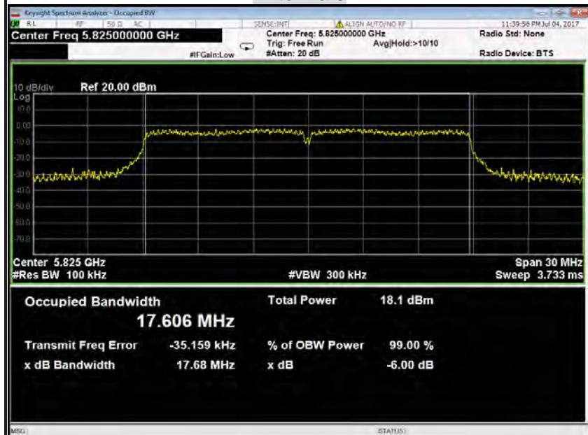
**IEEE 802.11ac 20 mode / 5745 ~ 5825MHz****6dB Bandwidth (CH Low)****Antenna 1**
