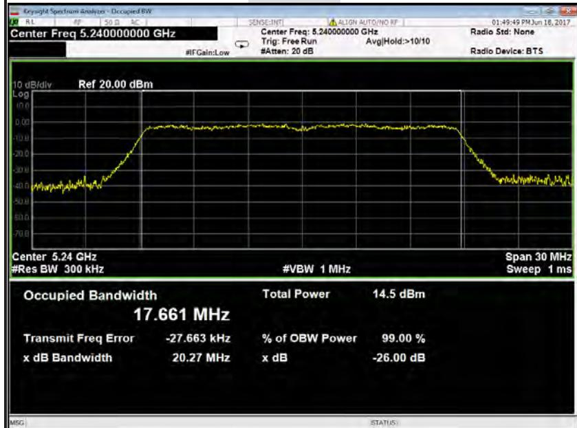
**IEEE 802.11n HT 20 MHz mode / 5260~ 5320MHz****26dB Bandwidth (CH Low)****Antenna 1**
