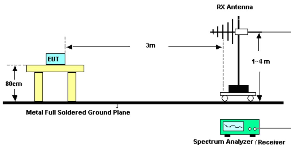
For radiated test from 1GHz to 18GHz
