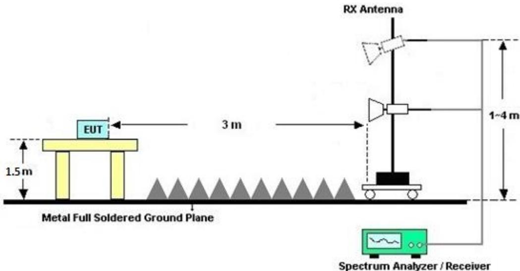
For radiated test above 18GHz
