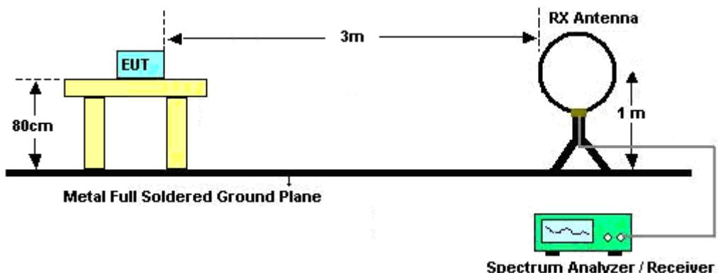
For radiated test from 30MHz to 1GHz
