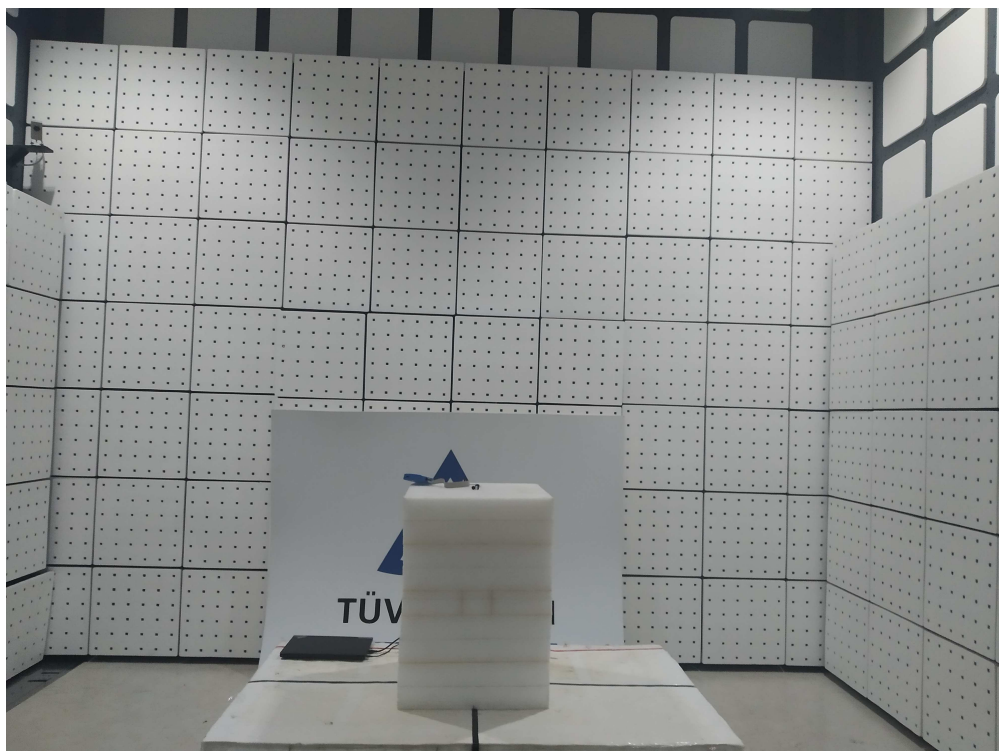
Photograph 2: Set-up for Spurious Emissions (Front View 2)
