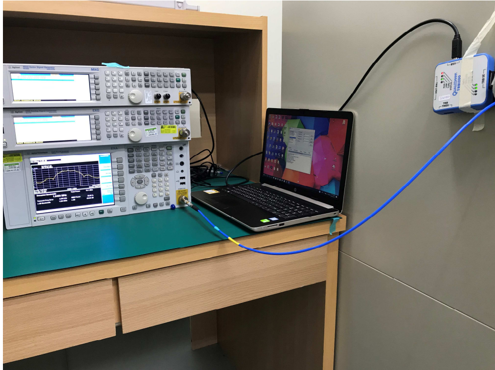
Photograph 8: Set-up for Conducted testing
