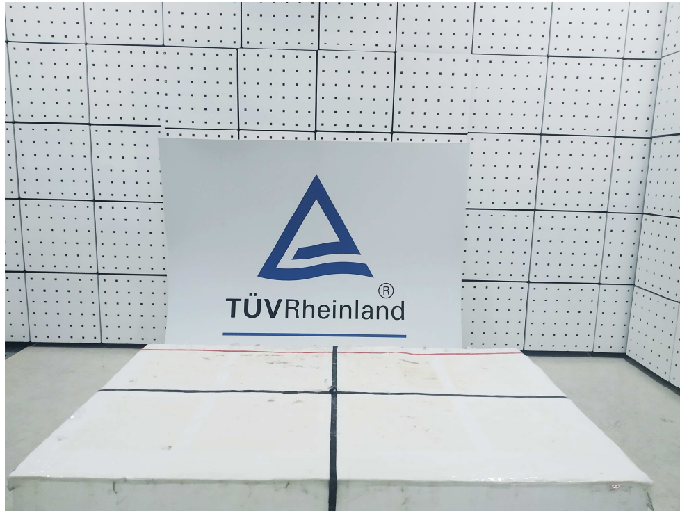
Photograph 1: Set-up for Spurious Emissions (Front View 1)
