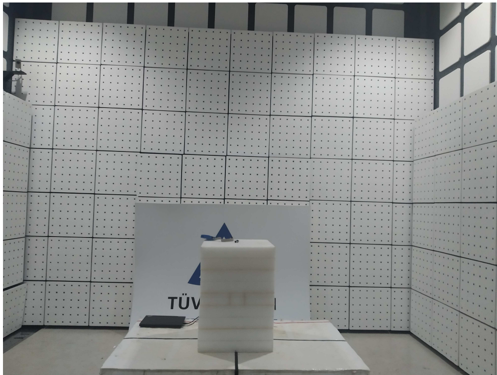
Photograph 3: Set-up for Spurious Emissions (Front View 2)
