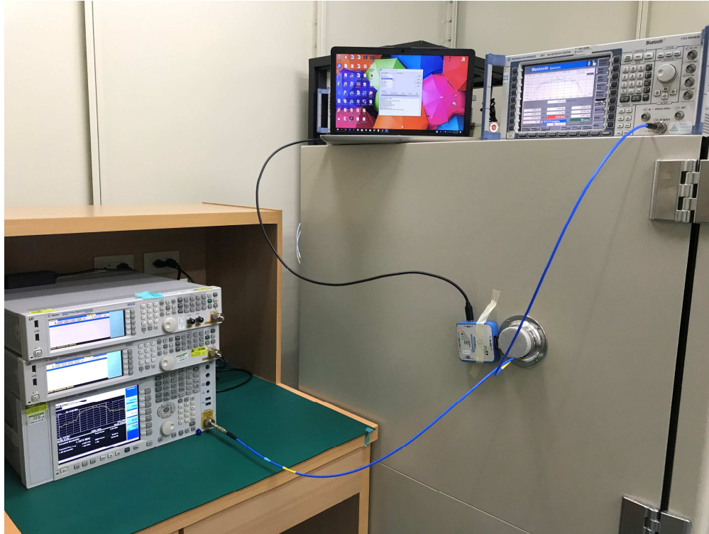
Photograph 8: Set-up for Conducted testing
