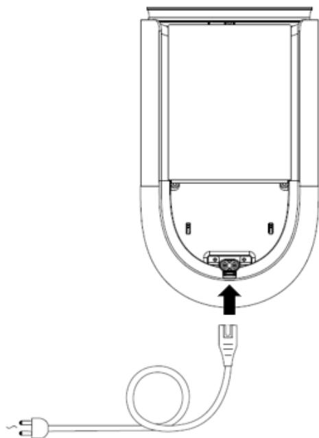
Unpack Beolab 8, connect it to the mains with the enclosed power cord and place it in its position.
