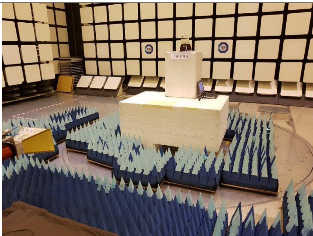
Band Edge Compliance (Radiated) Test Setup
