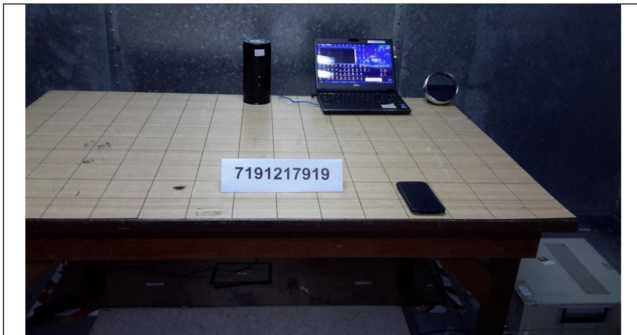
Conducted Emissions Test Setup (Front View)
