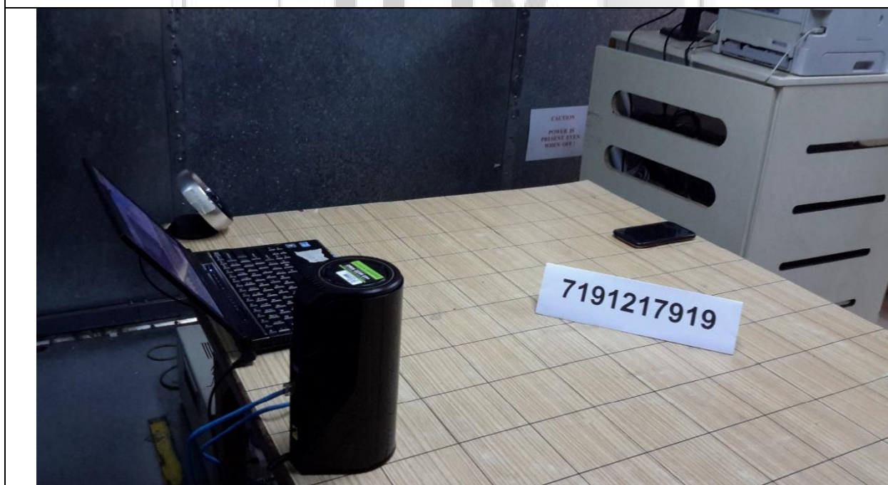
Conducted Emissions Test Setup (Rear View)
