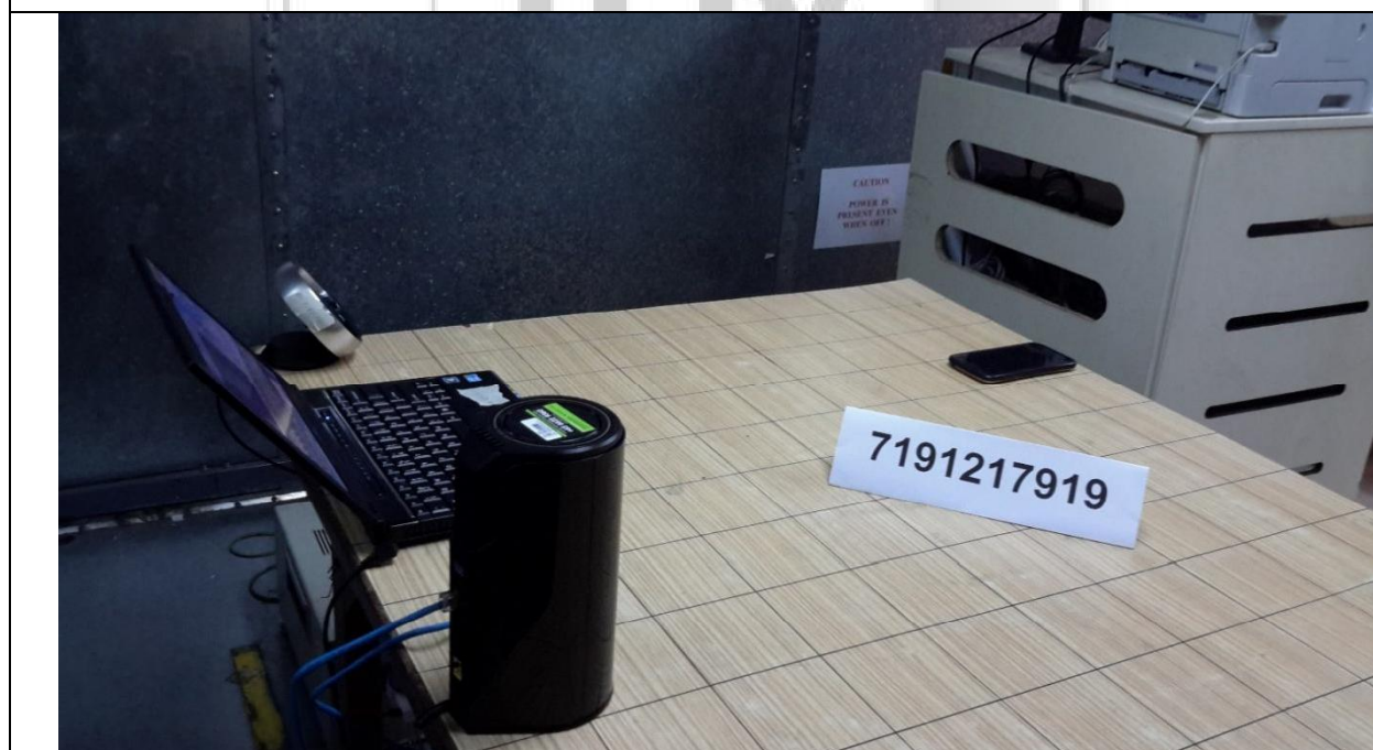
Conducted Emissions Test Setup (Rear View)
