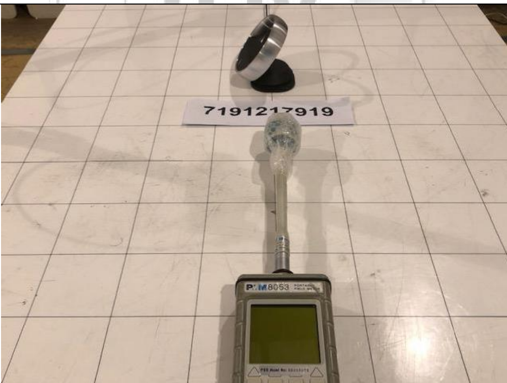
Maximum Permissible Exposure (MPE) Test Setup
