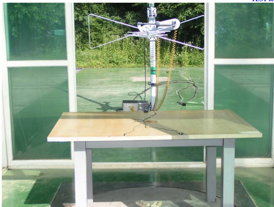
Radiated Emissions (FM receiving/Playback mode) -Z-axis View
