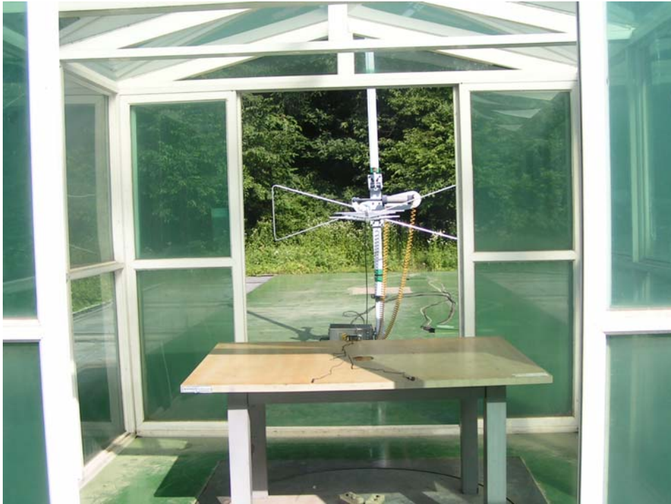
Radiated Emissions (FM receiving/Playback mode) X-axis View
