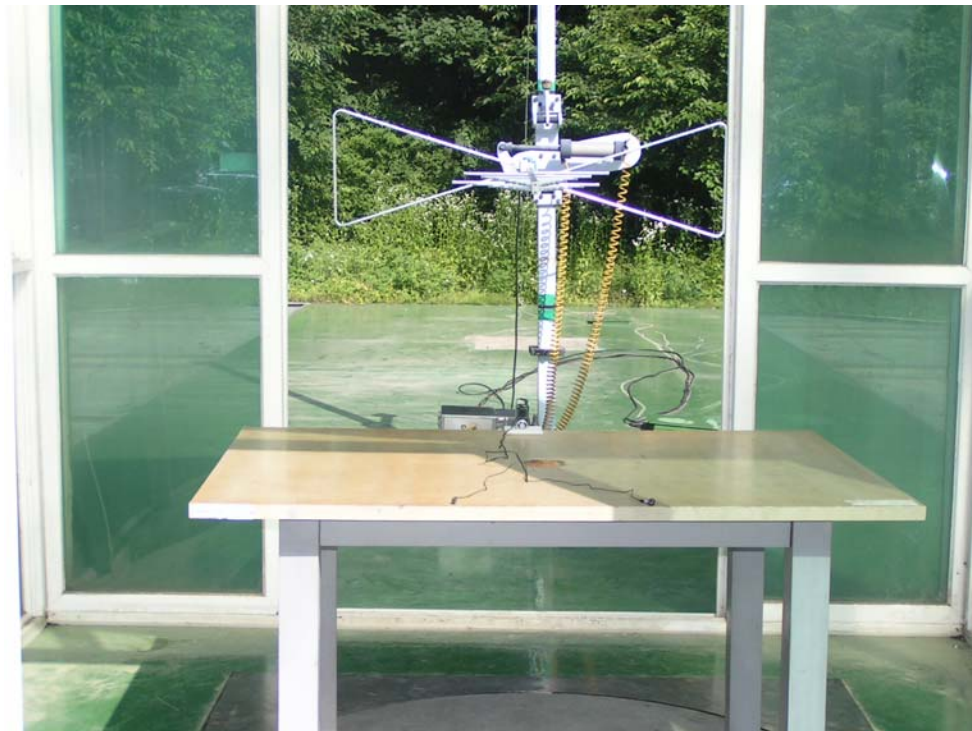
Radiated Emissions (FM receiving/Playback mode) -Y-axis View
