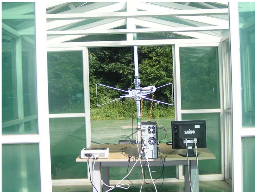
Radiated Emissions(File up/download mode)-Front View
