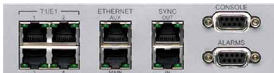
Figure 16 Primary front panel connectors (standard models)
