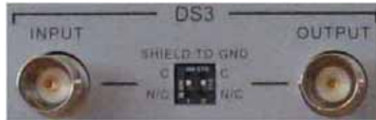
Figure 17 EX-5i-DS3 connectors and grounding switches
