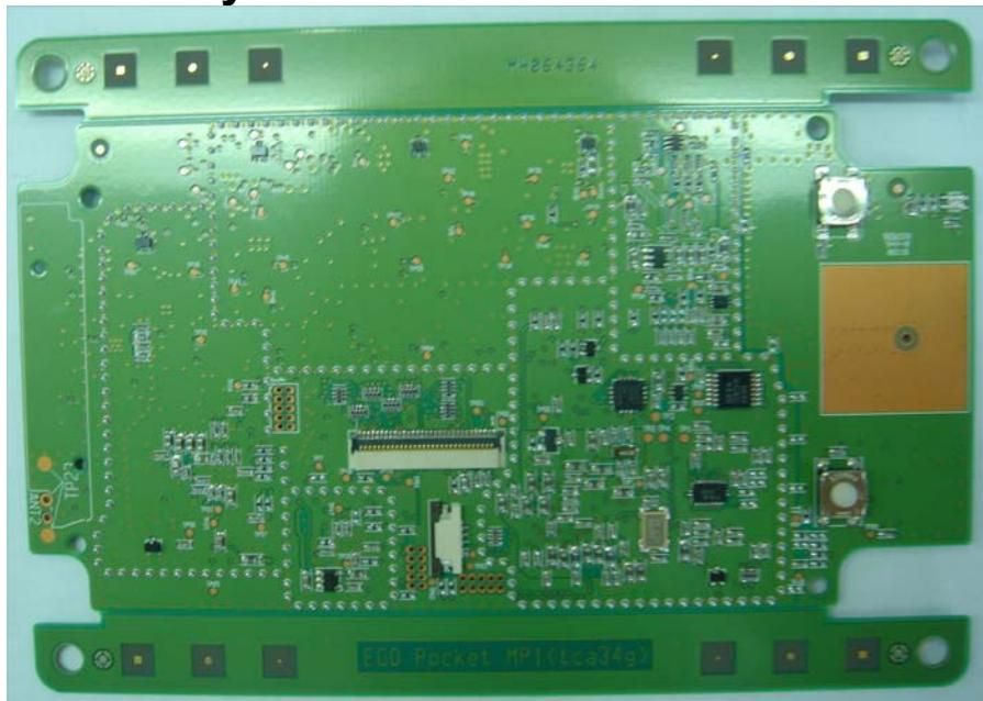
Note: Antenna ANT2 is not in this picture since it is mounted later in the production process after the shields have been mounted.
