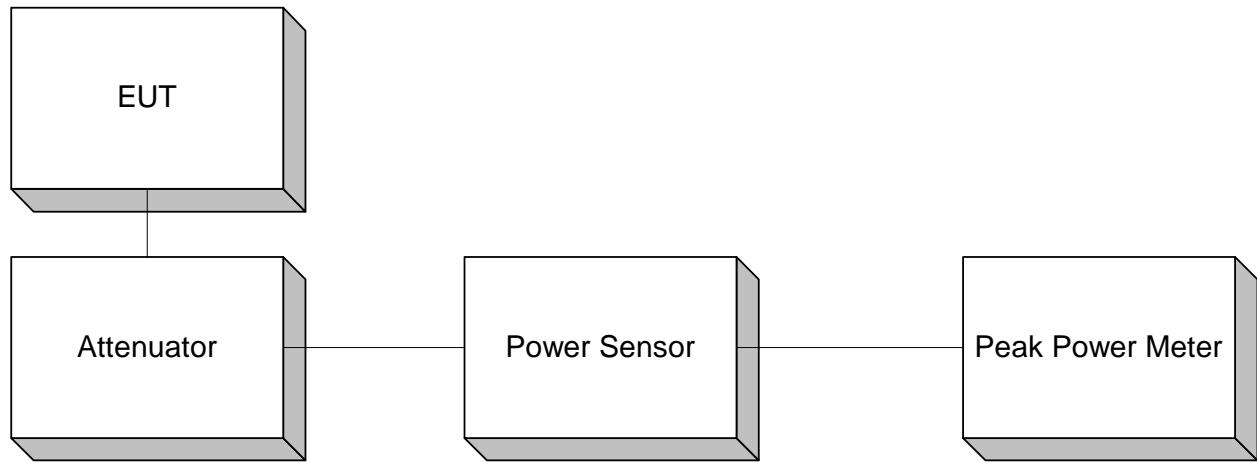
Note: A spectrum analyzer may be substituted for Peak Power Meter given that the measurement bandwidth is sufficient to capture the 60 dB bandwidth of the transmitter.
